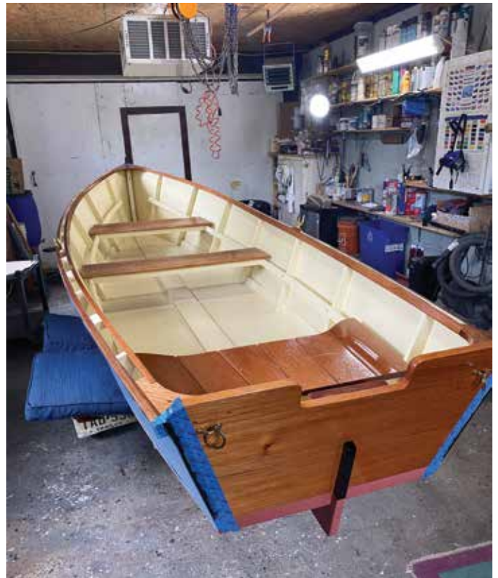
Below: Interior painted with finished seats installed.
