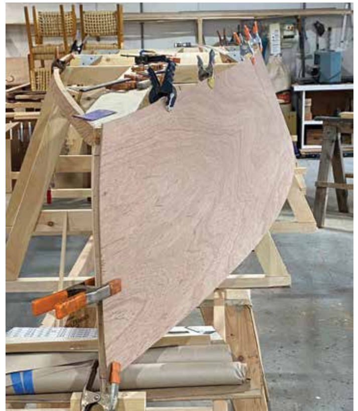
Bending on quarter inch plywood.
