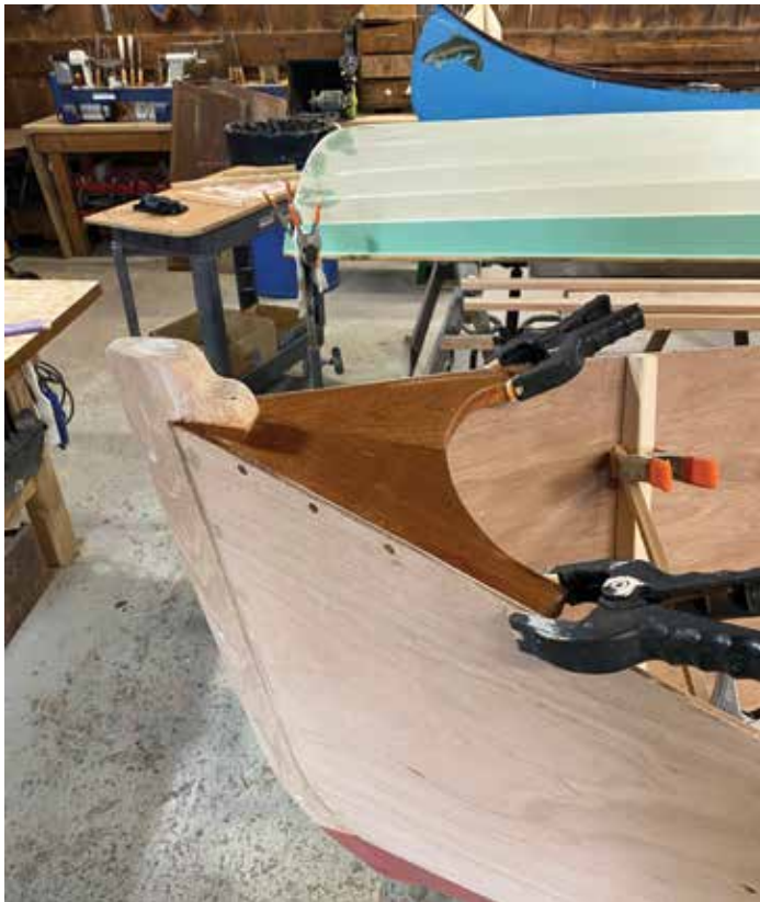
Below: Breasthook installed.
