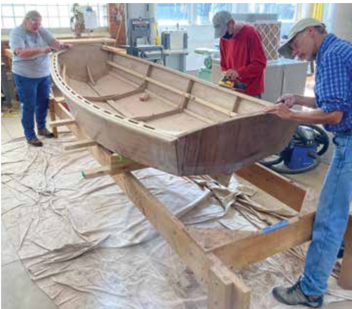
Right Top: The steamed white oak keel is bent into position by (L to R) Paul Jira, Steve Frye, Cindy Verbiak, and Ed Neal. Right Middle: Once flipped, the hull is trimmed and scraped of excess epoxy glue. Right Bottom: With the gunwale installed, floorboards became one of the final construction steps. Below: The final clean-up prior to painting was handled by (L to R) Cindy Verbiak, Dave Weglicki, and John Mikolich.
