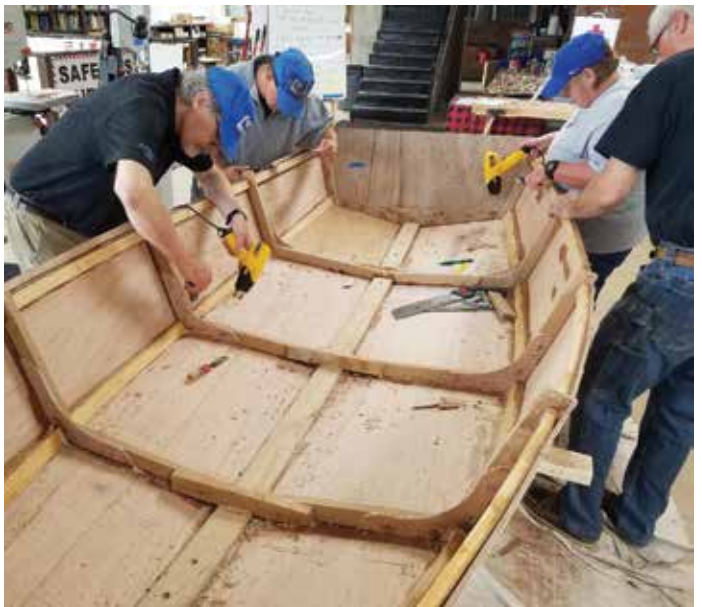
Right Top: The steamed white oak keel is bent into position by (L to R) Paul Jira, Steve Frye, Cindy Verbiak, and Ed Neal. Right Middle: Once flipped, the hull is trimmed and scraped of excess epoxy glue. Right Bottom: With the gunwale installed, floorboards became one of the final construction steps. Below: The final clean-up prior to painting was handled by (L to R) Cindy Verbiak, Dave Weglicki, and John Mikolich.
