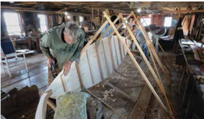
Top: With the basic components of the dory frame attached to the floor, the “skillet” is planed fair. (L to R) Brad Dimock, Cricket Rust, Graham McKay, Mick Fearn, Milford Buchanan. Bottom: Preparing to install the broad stroke. (L to R) Milford Buchanan, Graham McKay, Brad Dimock, Douglas Brooks.
