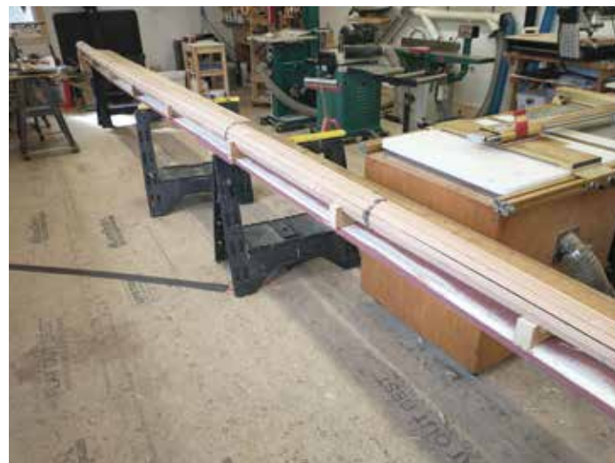
Left: Tapering the twelve staves for the main mast. Right: Dry fitting the twelve-stave mast.
