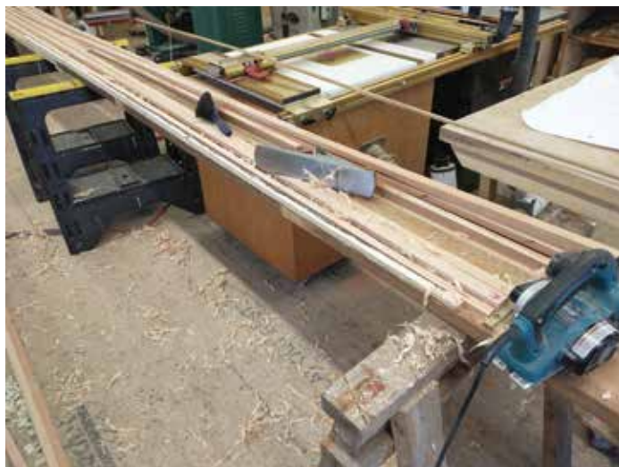
Left: Tapering the twelve staves for the main mast. Right: Dry fitting the twelve-stave mast.
