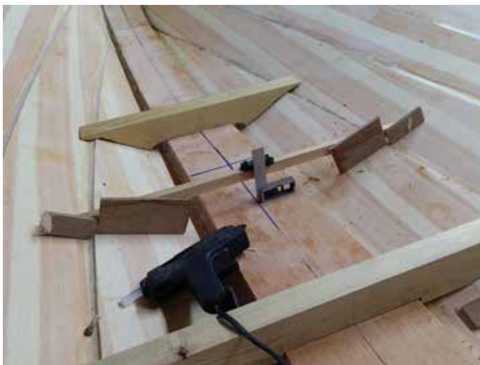
Hot gluing scraps to fit the floors.
