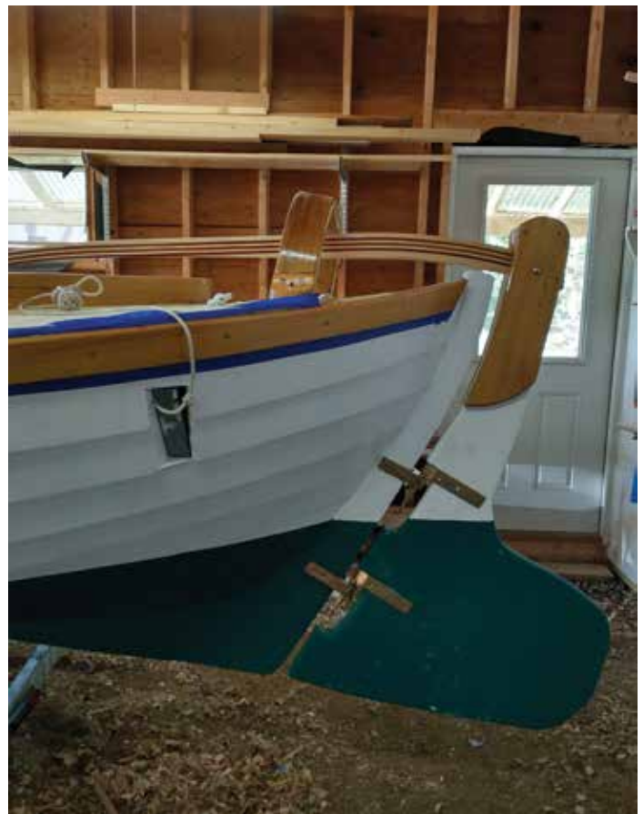
With the rudder hung, the tiller had to be designed to clear the coaming, and aft stemhead, while fitting under the mizzen arch.
