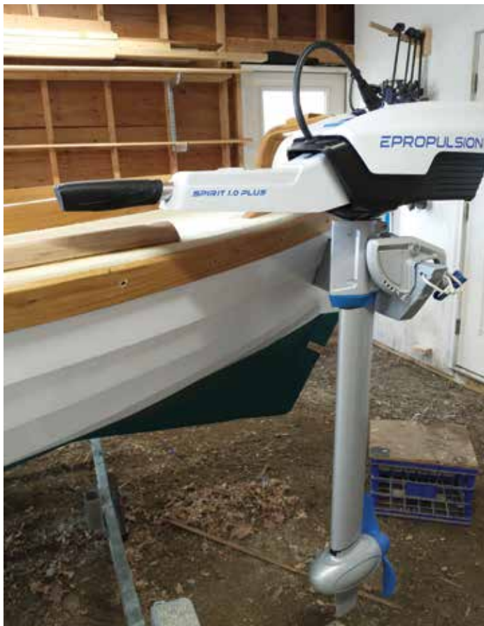
Checking the fit of the outboard on its sliding mounting bracket.
