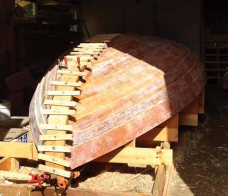
Hull, glass and epoxied with outer stem of laminated black locust.
