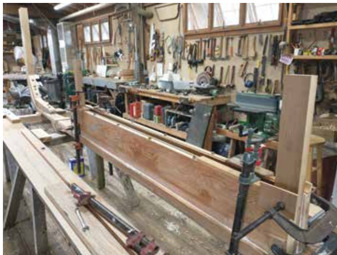
The centerboard box was made from two slabs of Cypress that was beaded on the bottom and let in to the keel. The bedlogs were bedded in 5200 and through bolted with bronze rod that were threaded at the ends to receive washers and nuts. After tightening, the thread protruding from the bolts were peened over so that the bolts can not work loose. The nut and washer on the bottom of the keel were given a wisp of cotton caulking soaked in red lead to prevent leaks.
