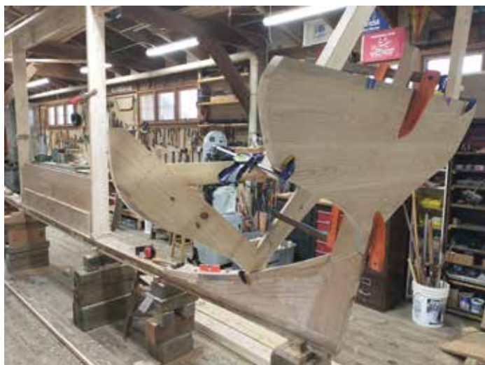
The white oak transom is being test clamped to the sternpost. This was made up from white oak tongue and groove planks that were then drifted with bronze rod.
