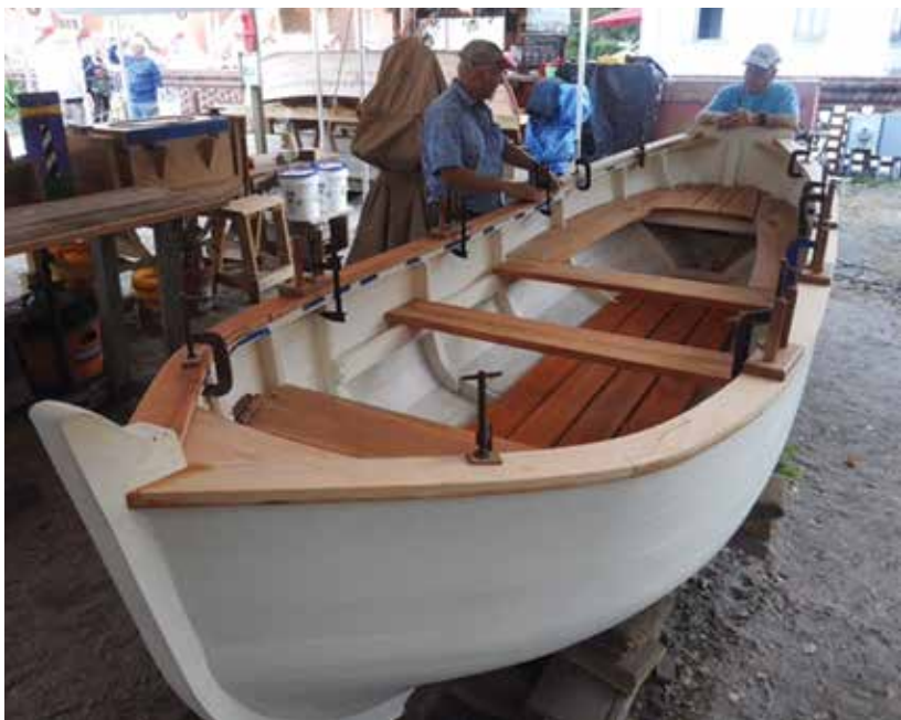
Below: Another yawl boat being built from the same authentic lines using carvel frame-first construction with sawn ribs.
