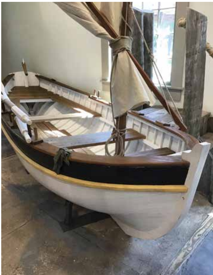
Left: 1760s British yawl boat of cypress built over molds with steamed ribs. Pictured on display at Mosaic, Jekyll Island Museum in Georgia.
