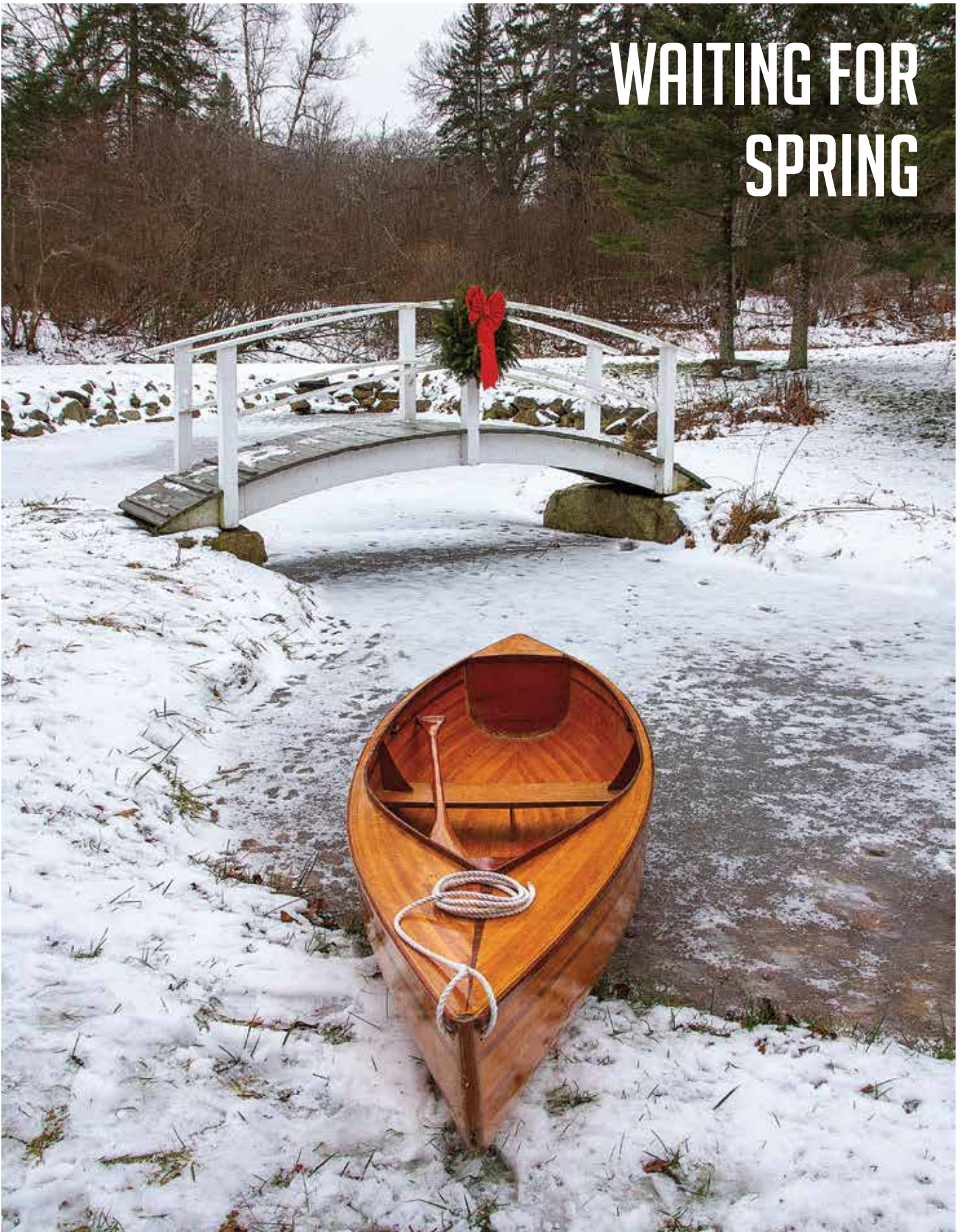
A 10.5 foot strip-built decked canoe designed and built by David Wyman. Photo by Rosemary Wyman.
