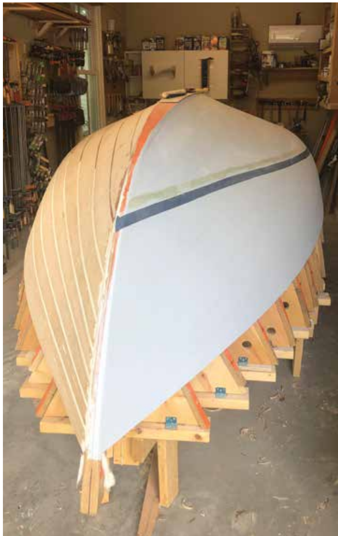
Above: Primer with Boot Stripe Below: Fairing the Keel Edge to the Garboard
