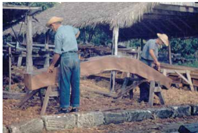
A boat being built at the Albury yard using the midship raising frame method. The man aft can be seen using the malleable lead bar used to pattern remaining frames.
