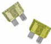
*fuse color depends on ampage ATO, ATC Style Fuse (blade fuse) Current Rating: 1 to 30 amps Voltage: 32 VDC max
