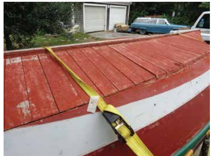
Figure 3: Herring bone bottom planking.
