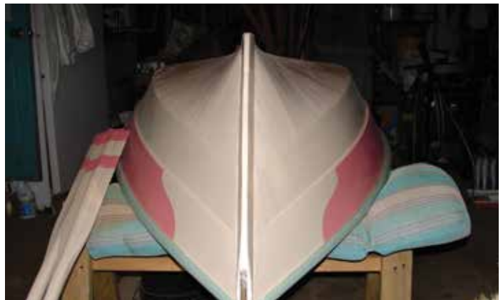
Figure 6: Luckily we did not have to disturb the bottom planking at the bow or the stern. This picture was taken before the brass rub strip was installed.
