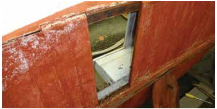
Figure 4: The first planking to be removed and the centerboard with its wooden pin removed.
