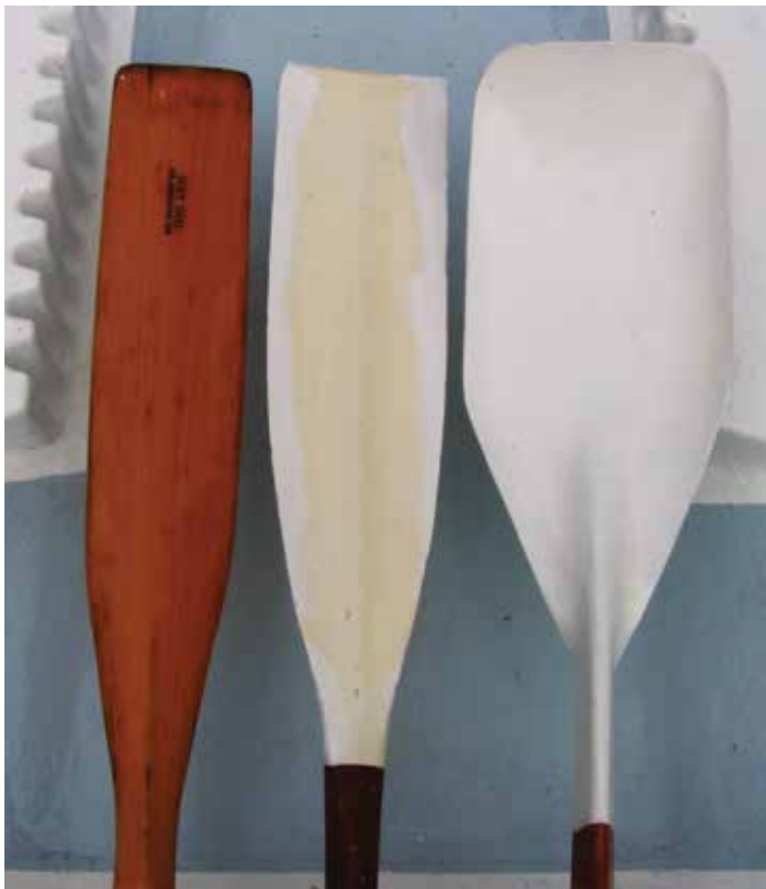
Left to right: Flat blade, 1955 Spoon blade, and the Turbo blade. Could it be that the material used dictates the narrow blades on the first two?
