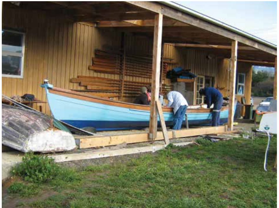
Thirty-four-foot replica of a six-oar NZ bay whaler, built by The Living Boat Trust, Franklin, Tasmania. Note the different oar lengths for the varying boat widths. It is "awkward" to row because the oars are too heavy, the rigging needs attention, and a regular crew would help.
