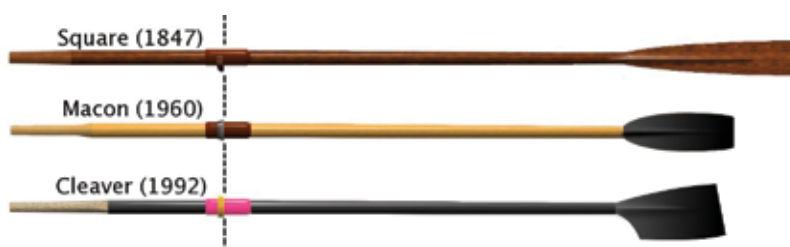
Diagram illustrating oar development over 170 years.
