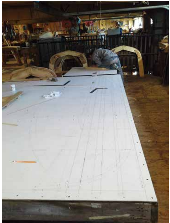
ADVANCED apprentice, Garrett Farchione has finished lofting for a Columbia Hershoff dingy.
