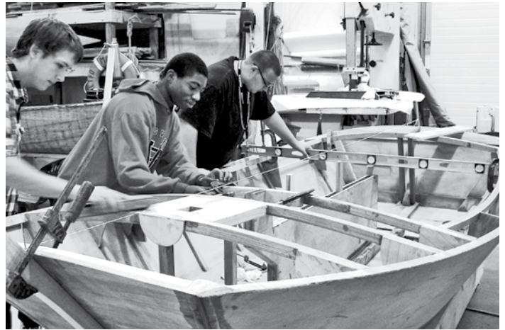
King plank and deck beams aligned
