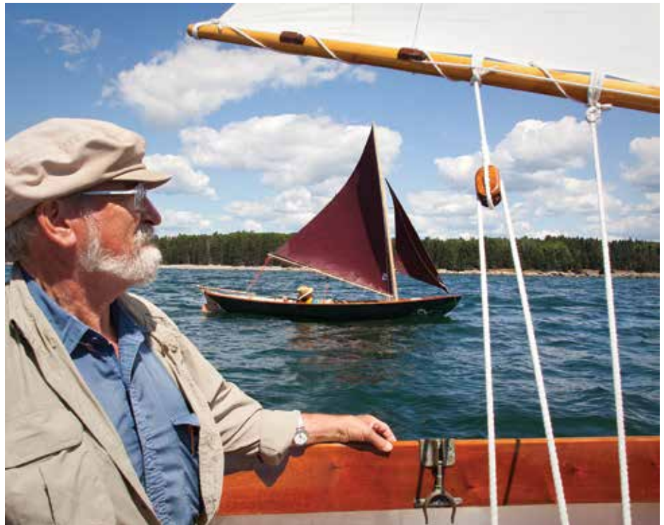
The Main Sheet made of rope and wooden blocks on the author's Canoe Yawl Island Lady with friend Steve Brown at the helm. Note that the lines are tied around the boom instead of using metal fittings.
