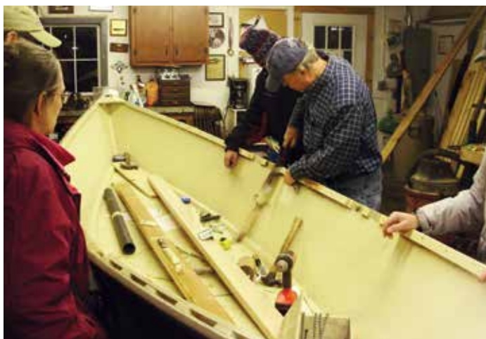
Friday was a full house, and we still managed to get some work done on the dory, along with hot dog eating and discussion. We glued and screwed the new inwales and installed blocking to hold the oarlock keepers.
