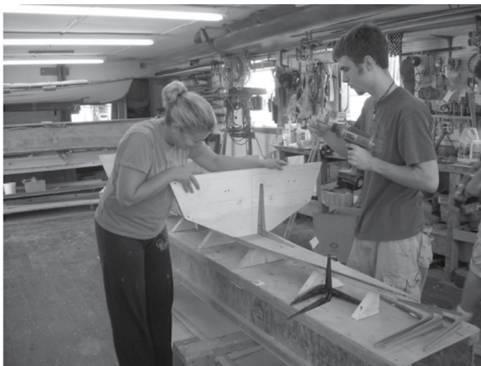
Placing the molds on the strongback
