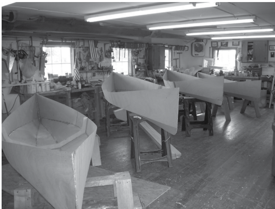
Four hulls assembled by the end of the first week
